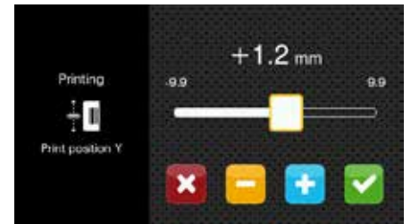
Print position Y Fast setup with a slider, fine setup with \pm keys
